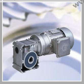
A variety of individual gear designs can be combined from few modules. The UNIVERSAL Worm Gear Unit SI features as standard foot mounting on three sides, B14 flanges on two sides and an output hollow shaft. Modules that enable various applications of the gear series are plug-in solid shafts, output-side bolt-on type flanges, torque arms Possible combinations of the modular system
