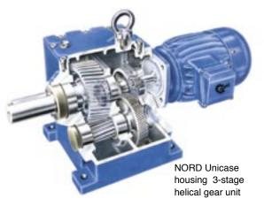
The wheel bodies are produced from forging blanks, the gearing is hardened, precision finished, rated for endurance strength, and conforms to calculations according to DIN 3990, Niemann and AGMA.
